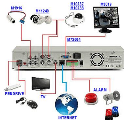
Fig.5.4 CCTV Camera Security System
