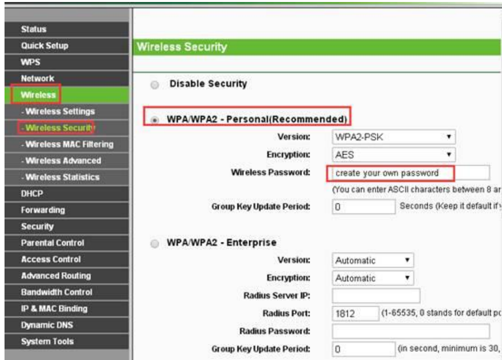
Fig. 3.20 Wireless Security Settings of a Router
