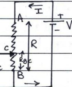
When slider C moves towards A, the length and hence resistance  $R_{BC}$  increases, so  $V_{BC}$  increases. When C moves towards B, resistance decreases so  $V_{BC}$  also decreases.
