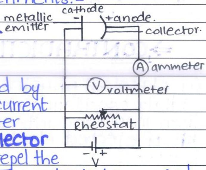
The voltage is varied by the rheostat until current through the ammeter decreases and **collector becomes -ve** to repel the ejected electrons. The potential is varied until **current drops to 0A**. This potential is known as **stopping potential** ( $V_0$ )
