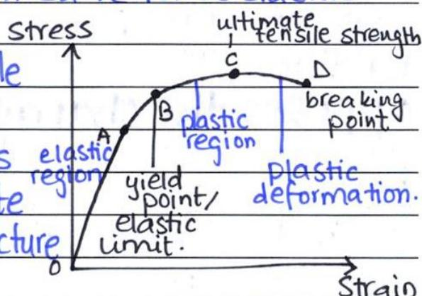
From the curve, we see that within the **elastic limit (stress  $\propto$  strain)** and body regains its original shape when force is removed. After elastic limit, is the region of **plasticity** where beyond the ITS body
