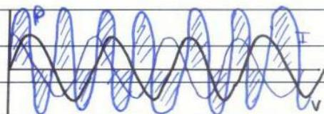
Q. No. 2 (x) → In RL series circuit, the current lags behind the voltage by angle  $\phi$
