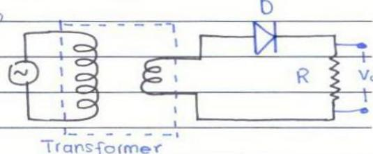
→ In negative cycle ( $T_{1/2}-T$ ), diode is reverse biased and no  $V_o$  is obtained at  $R$ .
