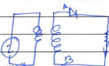
B so current passes through diode. It is forward biased. In negative half cycle no current passes through diode. as it is reverse biased.
