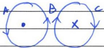
Since in two wire carrying current in opposite direction the field will be stronger at point B so since force acts from high field to low field so magnetic force ( $F = ILB \sin\theta$ ) will act from B to A and B to C as a result wires will repel.
