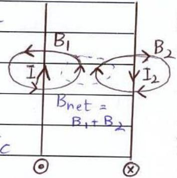
Whereas, the magnetic field outside the wires is weak. For this reason, the force will be directed from between centre of wire to outside. Hence, the wires repel each other.
